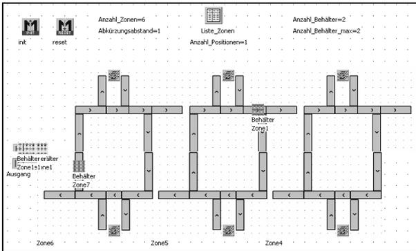
Figure 8: Zone-picking simulation module in eM-Plant
