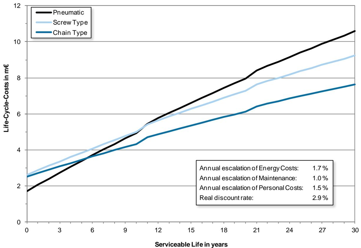
Fig. 6: Life Cycle Costs of different kinds of ship unloaders
