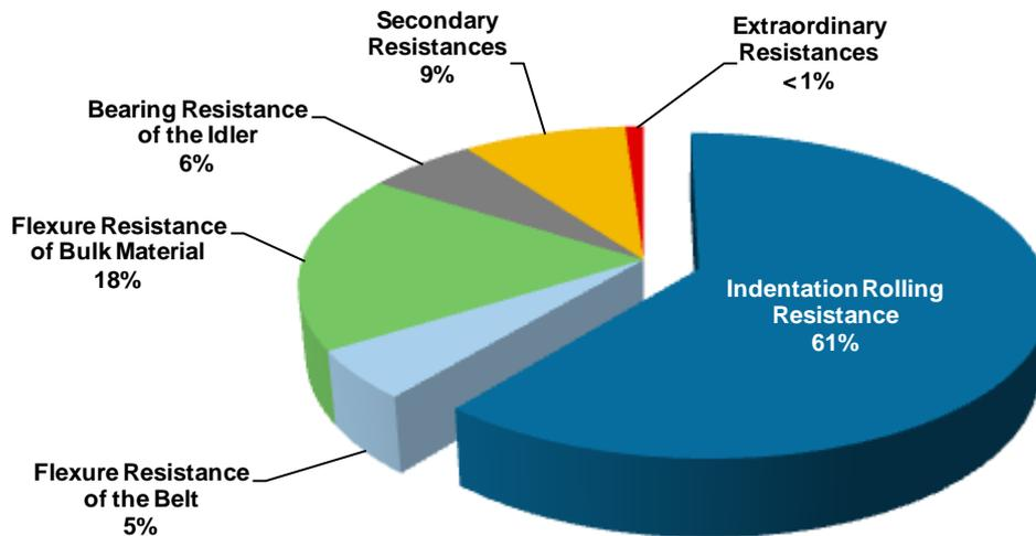
Fig. 5: Percental distribution of motion resistances of a long-distance horizontal belt conveyor [17]
