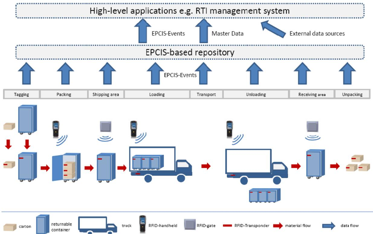
Fig.1 A framework for EPCIS-based tracking and tracing
