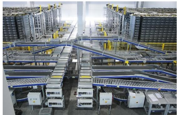
Fig. 1. Example of a stationary material handling system from SSI Schäfer.
