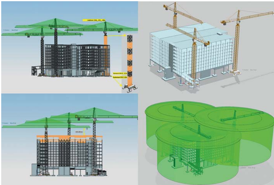
Fig. 4: 4D tower crane planning – practical examples (source: Max Bögl GmbH)
