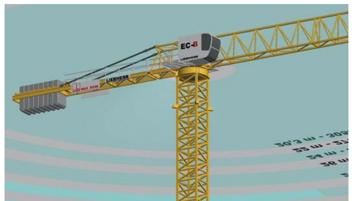
Fig. 2: 3D tower crane modelling using the tower crane deployment planner
